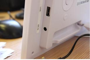
Plug the power cable into the DC IN socket on the right side of the frame. Plug the cable into the mains and switch on at the socket.
